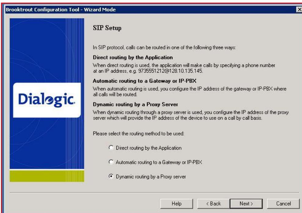
In the SIP Setup screen you will have three choices. The babyTEL SIP trunk uses a server for proxy and registrar functions. Choose **Dynamic routing by a Proxy server** then click **Next**.
