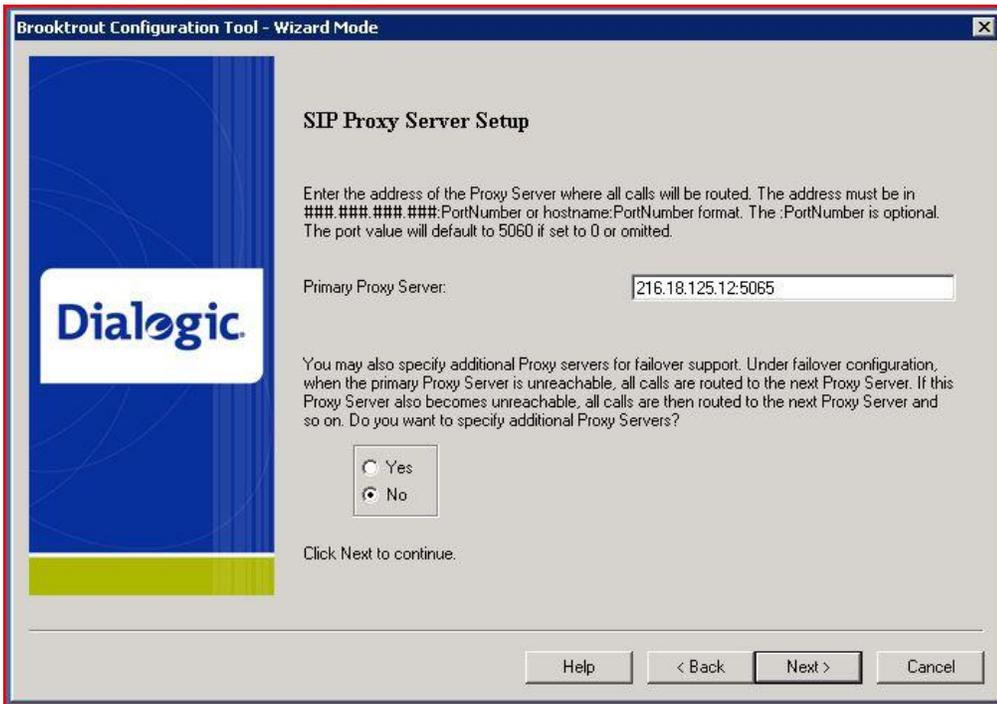
The IP address of babyTEL's proxy server is 216.18.125.12 and it uses port 5065 for communications. Enter **216.18.125.12:5065** in the **Primary Proxy Server Field** of this window. Choose **No** as to whether or not you want to specify an additional proxy server.
